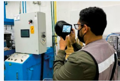
Finding air leaks in Juarez
