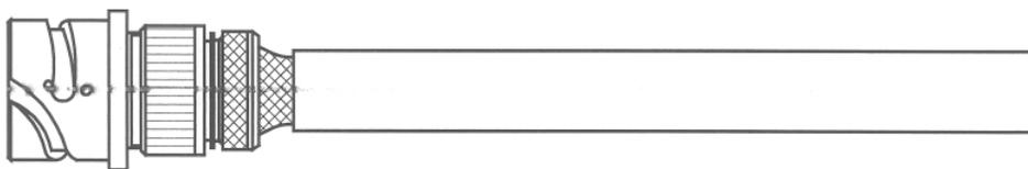
**Figure 33. Installed Nut**
