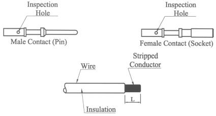
Figure 11. Stripping and Crimping Operation
