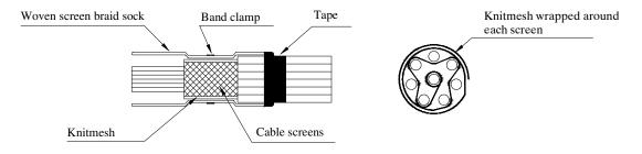
Figure 16. <u>Installation Of Knitted Mesh Braid</u>
