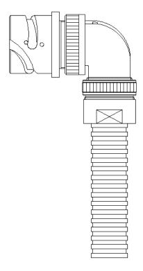
Figure 28. Example of Finished Assembly (90 Degree Elbow)
