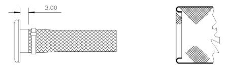
Figure 20. <u>Termination of Braid Sock to RFI Adaptor</u>
