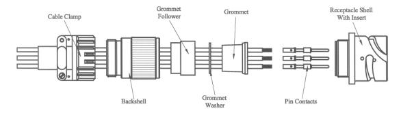
Figure 4. <u>Individual Wire Termination Procedure (Shown on Receptacle Connector)</u>
