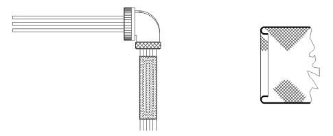
Figure 18. Slide Parts Along Cable in Correct Order
