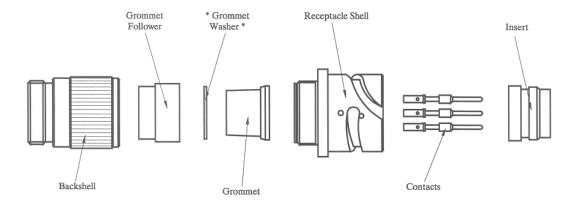
Figure 3. <u>Exploded View of a Typical 'Plug' Connector</u>
