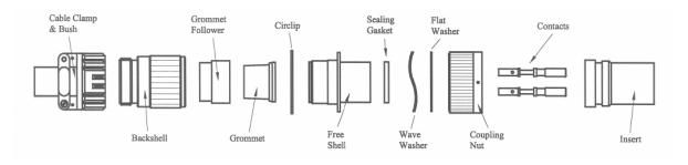
Figure 2. Exploded View of a Typical 'Plug' Connector
