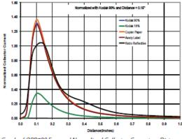
Graph of OPB700 Focused Normalized Collector Current vs. Distance to a Reflective Surface.
