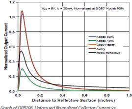
Graph of OPB706 Unfocused Normalized Collector Current v. Distance Reflective Surface.
