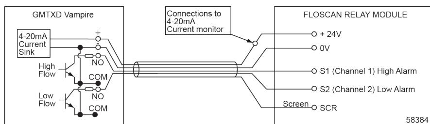
The Platon Vampire d.c. powered flow transmitter (see OMM1033) can be powered from the Floscan relay module, and the alarm outputs used to drive the relays. Note that current sensing for the flow analogue output must be in the 24V line.
