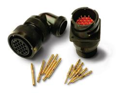
Circular, reverse bayonet lock connector range for signal and power, derived from MIL-DTL-5015 and VG95234. The range includes 8 shell sizes (18 to 40), 9 contact arrangements (7 to 60 ways) with contact sizes 16, 12 and 8 AWG.
