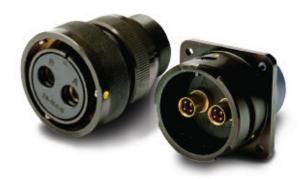
The 1 to 11 module (containing multi-pole contacts), Signal/High Speed Data Connector is based on the popular ABCIRP, MIL-DTL-5015 and VG95324 bayonet lock connector. This Rugged and reliable product range is shock and vibration tested to BSEN61373 Cat 1. Class A and has an endurance of minimum 2000 mating/unmatings. Crimp removable contacts make assembly and maintenance easy.
