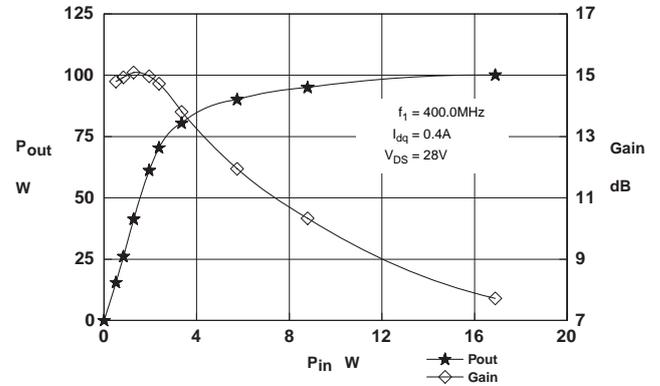
**Figure 2 – Power Output & Gain vs. Power Input.**
