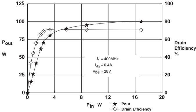
**Figure 1 – Power Output and Efficiency vs. Power Input.**
