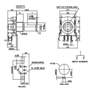
MODEL EN11-VNM (Side Adjust, without Switch, Threaded Bushing)
