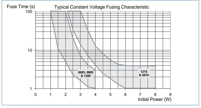
Note – actual fusing characteristics depend on mounting conditions. Reference conditions are FR4 substrate with 35• m (1oz) copper, pad and track width as follows: 0603 – 1.5mm, 0805 – 1.7mm, 1206 – 2mm, 1210 – 2.9mm, 2010 – 3mm.
