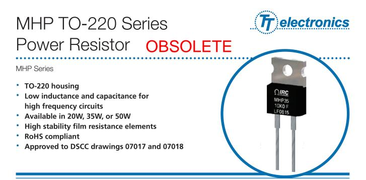
IRC's MHP series resistors satisfy demanding applications for accurate and stable power resistors housed in the convenient TO-220 case. The resistance element is isolated from the mounting tab by an alumina ceramic layer, providing very low thermal resistance and ensuring high insulation resistance between terminals and tab. The non-inductive design makes these products especially useful in high frequency and high speed pulse applications.
