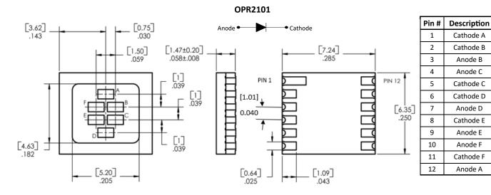
DIMENSIONS ARE IN INCHES AND [MILLIMETERS].
