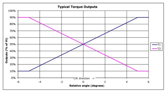
Different output signals can be easily configured by BI. Contact factory for details.
