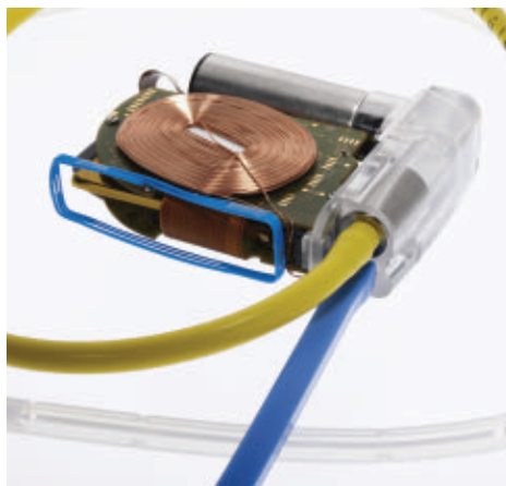
The alfa pump employs a battery-powered, low-flow pump and a set of two catheters to transfer fluid to the bladder.
