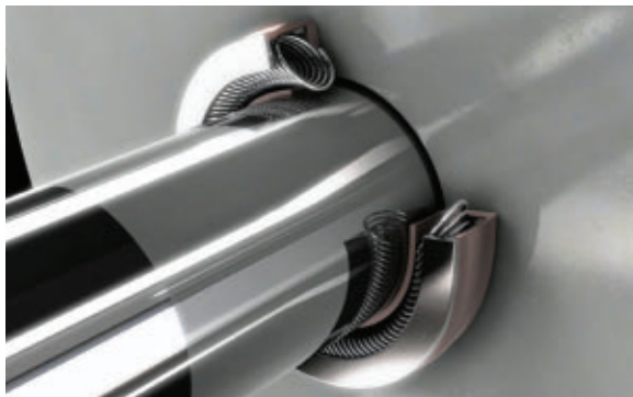
The addition of the spring-energized seal to the alfapump design reduces device power consumption by 40% and increased battery life by 20%.
