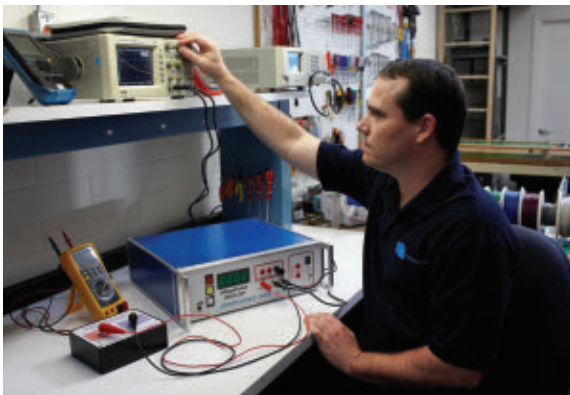
Hipot, surge, and other hazardous tests should be separated from the normal workflow to protect other personnel.
