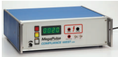
CMs use surge testers based on IEC 60601 for verification testing.
