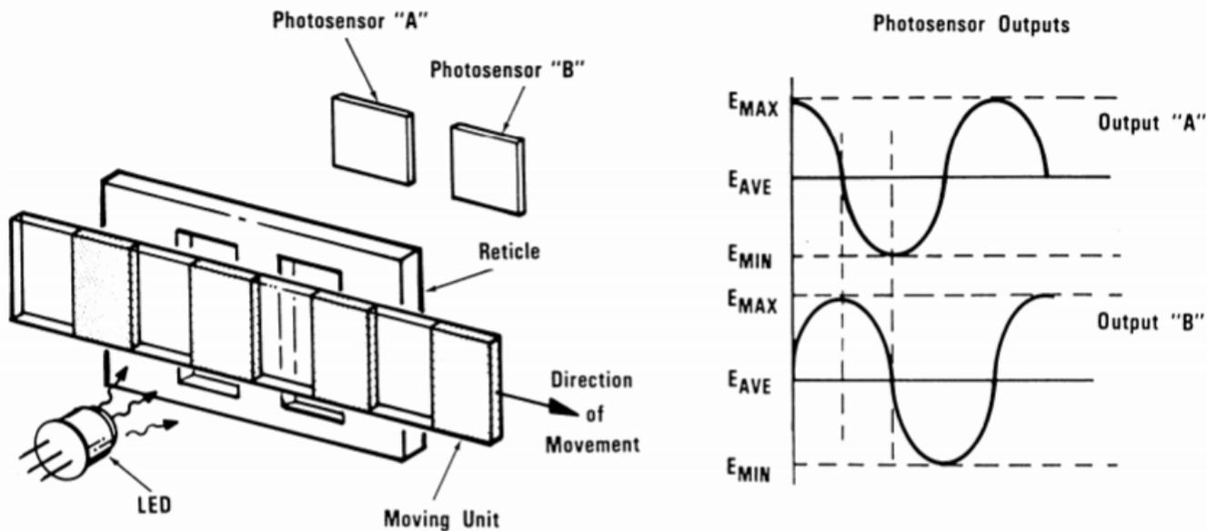
The output from photosensor “A” rises 90° ahead of the output from photosensor “B” indicating that the moving unit is moving to the right. If the moving unit were moving to the left, the output from “B” would be 90° ahead of “A”. For more information on dual channel encoding refer to Application Bulletin 203.
