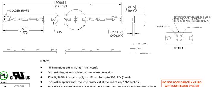
To add solder bumps to the cut sections, the X-Acto\* #16 scoring blade works very well to expose the copper contacts. Caution should be exercised so as not to remove the copper coating.
