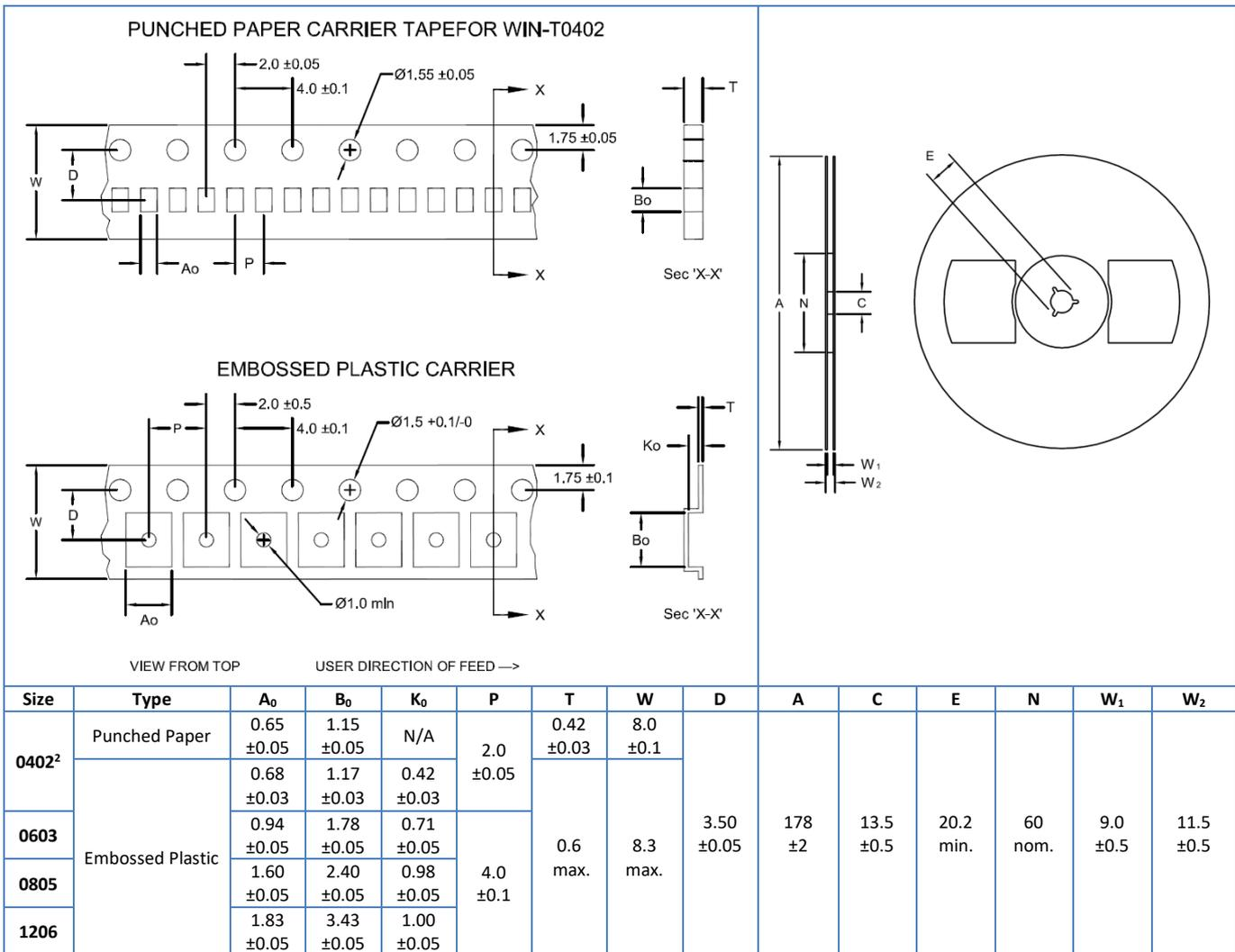
Note 1: Dimensions and materials conform to EIA-481 standard.
