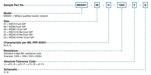
Standard termination is gold plate. Contact factory for optional 60/40 Sn/Pb hot solder dip finish.
