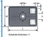
Dimension d = clearance between exposed conductor and exposed steel substrate. Fixing hole is located centrally except on WSHR1/2 where the dimension from the edge by the terminations to the mounting hole centre is 16.68mm.
