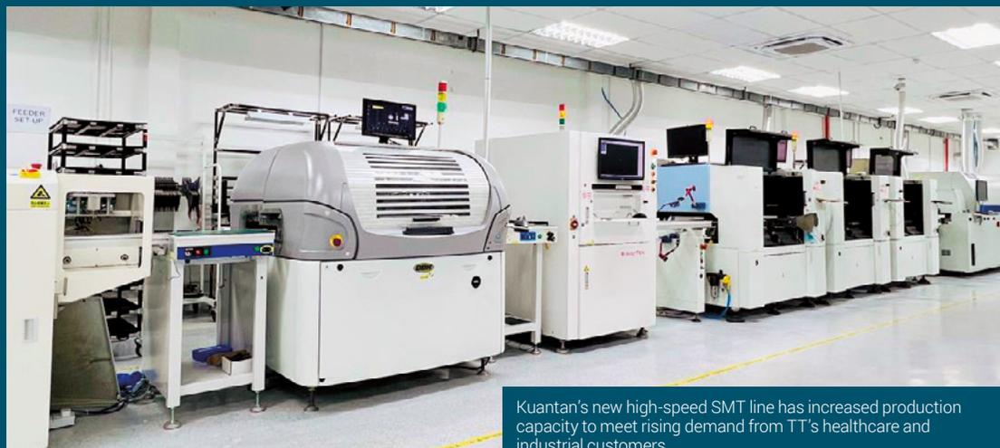
Kuantan's new high-speed SMT line has increased production capacity to meet rising demand from TT's healthcare and industrial customers
