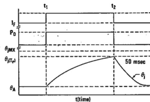
**Example:** A single 1A pulse 100 sec wide is applied to an OP136. What will the junction temperature be at the end of the 100  $\mu\text{sec}$  pulse?
