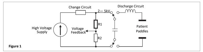
In this circuit R1 is a high value resistor, normally in the range 5M to 50M, which, together with a commodity chip resistor R2, forms a potential divider for voltage feedback.
