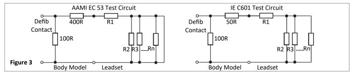
The proportion of the total defibrillation energy received by a protection resistor depends on its ohmic value, and the highest value consistent with monitor function should be used to minimize this. There is also a variation depending on which test circuit is used, and, in the case of IEC601, on how many leads are in the leadset.
